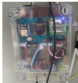
Figure 9. All components inside waterproof case
