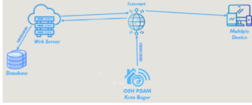
Figure 4. Working principle of proposed web user interface
