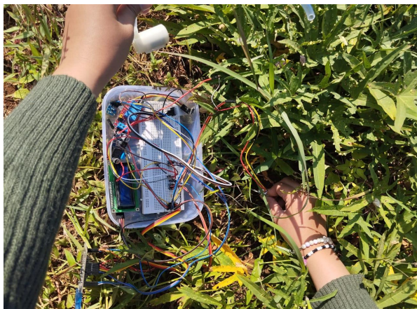
Figure 1. Prototype Setup for Data Acquisition in Sweet Potato Field, Halimpu Village, Cirebon Regency.
