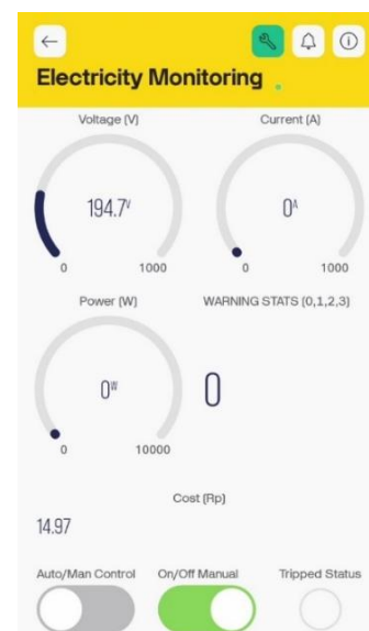
Figure 5. Dashboard platform monitoring system
