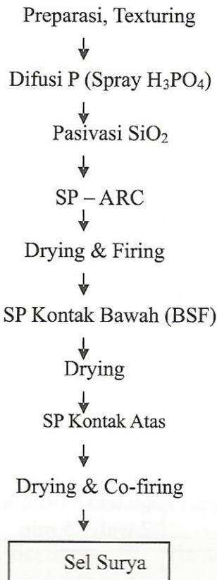
Gambar 1: Tahapan Proses Sel Surya
